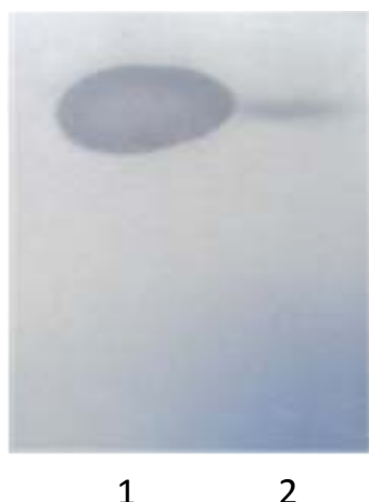
Fig. 5. Zymogram of the enzyme after incubating the native-PAGE gel for 12 h at 37°C in the substrate. Column 1- A standard strain with a molecular mass of 43 kDa ( Bacillus thermocatenolatus lipase in recombinant pichia pastoris ). Column 2- Lipase activity of Pseudomonas L.M. was visualized as a clear band on the tributyrin agar plate.
