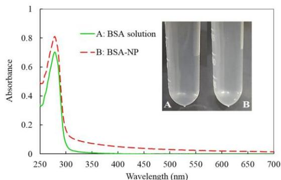
**Fig. 5.** UV-visible spectra and appearance of BSA solution, before (A) and after (B) nanoparticle formation.
