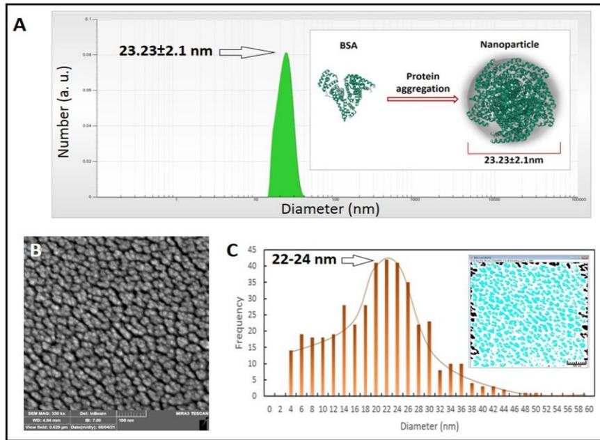
**Fig. 1.** Size analysis of BSA-NP. A) Size distribution in colloidal solution by DLS analysis, B) FESEM micrograph of dried BSA-NP and histogram of their size distribution (C) analyzed by imageJ software.
