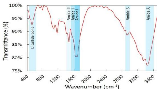
**Fig. 4.** Confirmation of protein characteristics of BSA-NPs by FTIR. Blue regions are indices of proteins FTIR spectra.
