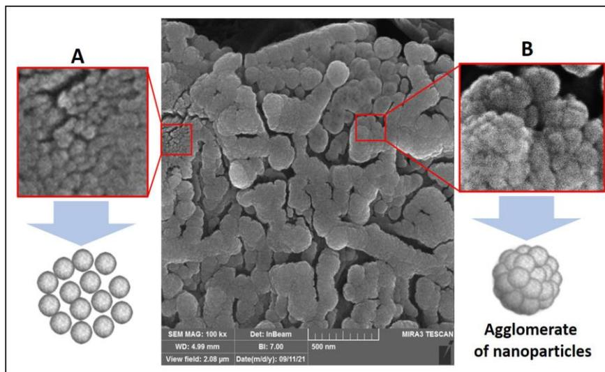
**Fig. 2.** Morphological analysis of BSA-NPs using FESEM. A) Small aggregation of NPs. B) Larger agglomerated of BSA-NPs.
